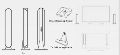
1. Place the light bars on both sides of the table or mount them to the TV screen with the mounting bracket.
